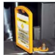
Use Frame at Oil Fill Points
