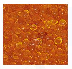
The clear view 360 degree design makes it easy to inspect the saturation of the color-changing silica gel from a distance. The inert silica gel turns from gold to dark green to visually indicate the adsorption of moisture and confirm the breather is getting the job done.
