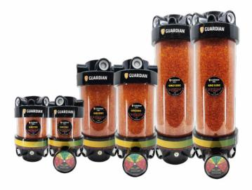
check valves prevent exhaust air from depleting the desiccant while shielding against volatile fumes and splashing fluids, while compound indicating gauges provide an accurate indicator for filter conditions.
